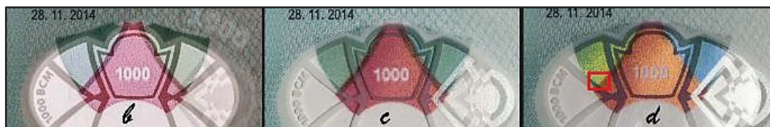
Fig. 290b — viewed in transmitted light; 285c — reflected light at 45°: both elements appear similar in colour; 285d — reflected light at 0°: left element golden, right element blue
